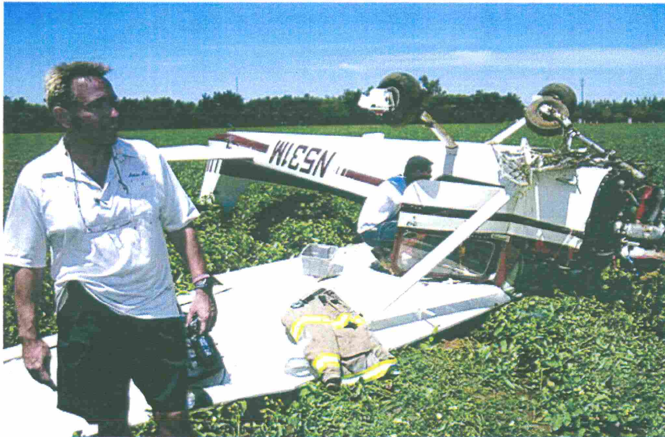
This Cessna 150 crash landed in a tomato field and was damaged beyond repair after a hawk shattered the windshield during approach to a California airport, 20 July 2007. Photo, Matthew Henderson.
